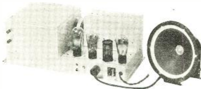
THE RECEIVER AND DYNAMIC SPEAKER CHASSIS, AS REMOVED FROM THE CABINET. NOTE THE COMPLETE SHIELDING OF ALL SCREEN-GRID R.F. TUBES AND CIRCUITS; ALSO THE AUTOMATIC LINE-VOLTAGE REGULATOR, FUSES, AND METHOD OF CONNECTING THE SPEAKER
