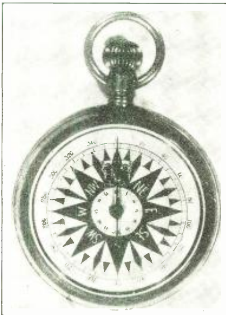
THIS SHOWS THE TYPE OF STOP-WATCH, HAVING THE DIAL DIVIDED IN POINTS OF THE COMPASS, WHICH IS USED TO FACILITATE THE TAKING OF BEARINGS WITH THIS BEACON
